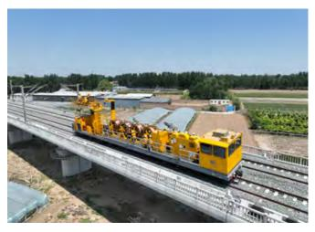
China Railway's self-developed contact wire assembly vehicle with constant voltage.
